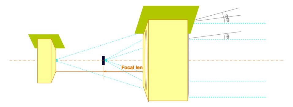
Efficiency decreases when θ or E<sub>photon</sub> increases => to increase either the efficiency or the upper energy cut-off threshold, one must increase the focal length
