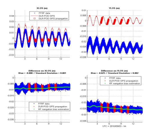
The good performance of the CNES onboard navigation filter is confirmed in the last figure, which shows the first real-time estimation of the relative position of MANGO with respect to TANGO. The position noise is less than 3 cm along track (X) and less than 12 cm in nadir direction (Z), compared with the GPS. The relatively poor cross-track (Y) precision of 6,4 m is unsatisfactory, but is expected to improve significantly once the filter parameters have been tuned.
